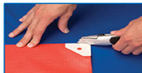
Cut off loop if not needed
